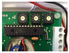
As you can see above there are 3 dials, dial 1 on the left is **NOT** needed for device numbering. Dial 2 and 3 are used for your device numbering, as you can see dial 2 is set to 0 and dial 3 to number 3. This makes the device number 03. to set a device to number 20 for example dial 2 would be set to 2 and dial 3 set to 0.
